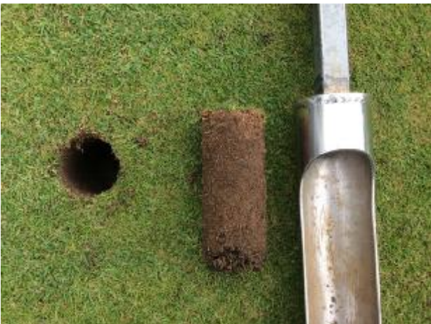
Figure 17: Inspection of the soil profile on the green at Leys shows some accumulation of organic matter near the surface.
